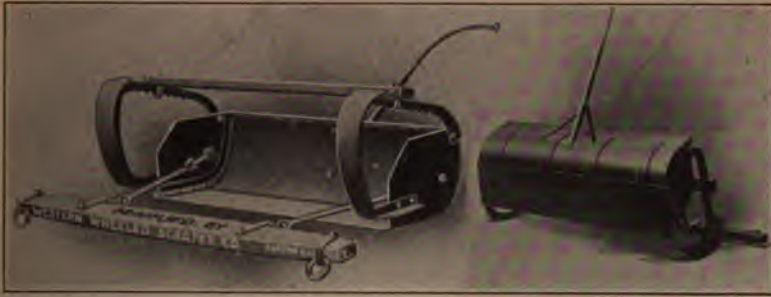
Buck Scraper ready to Load. Figure 4.
